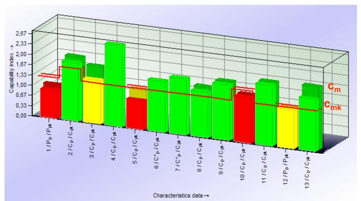
"capable machine" means: all characteristics are capable
